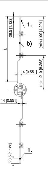
for 2-point latch PHZ 6-503, with lock cover and flat rods with rollers
